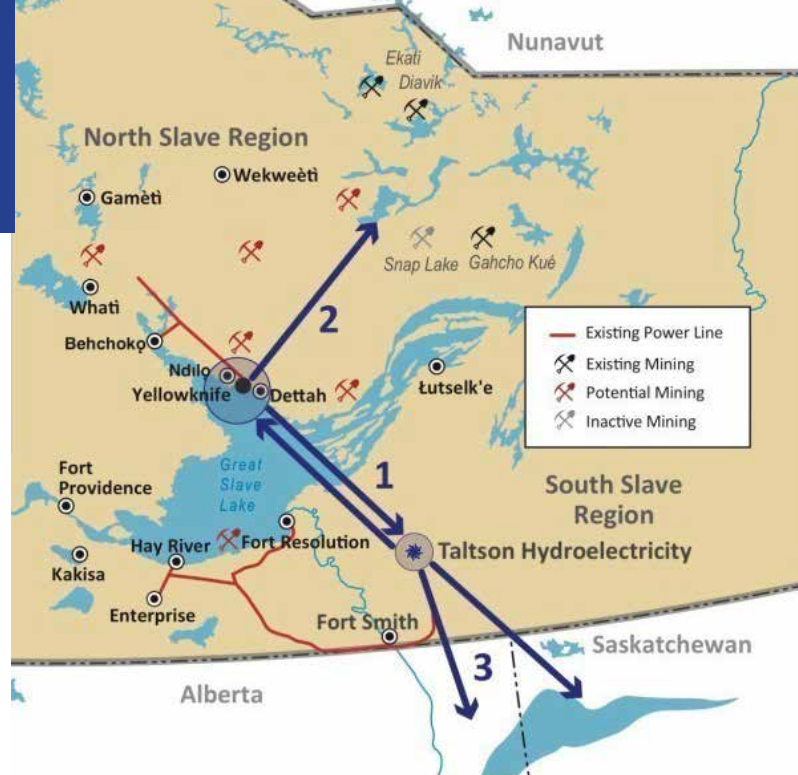
Proposed Taltson Hydroelectricity Expansion showing the 3 planned project phases. Map courtesy of Government of Northwest Territories Infrastructure
